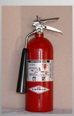
A CO<sub>2</sub> may be ineffective in extinguishing a Class A fire because it may not be able to displace enough oxygen to successfully put the fire out. Class A materials may also smolder and re-ignite.
