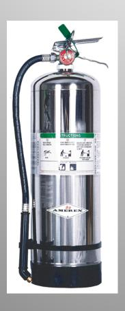
These fire extinguishers work on the principal of saponification. Saponification takes place when alkaline mixtures such as potassium acetate, potassium citrate or potassium carbonate are applied to burning cooking oil or fat.
