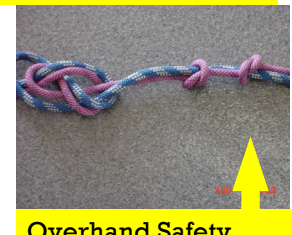
Overhand Safety Knot
